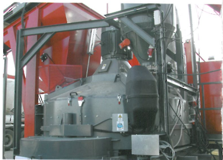
The powerful counter flow mixer has a cycle time of just 1 ½ - 2 minutes
